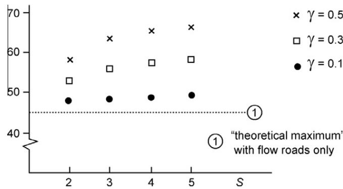
Fig. 2. The relative number of fatalities for four scales of traffic calming and for three levels of effectiveness compared to the initial road network.
