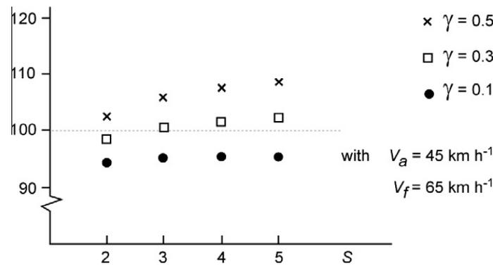
Fig. 3. The relative values for travel time per grid cell for four scales of traffic calming, three levels of effectiveness, for speeds of 65 on flow roads and 45 km h<sup>-1</sup> on access roads, compared to the initial road network with diffuse flows and without traffic calming. Source: Van Langevelde and Jaarsma (2009)
