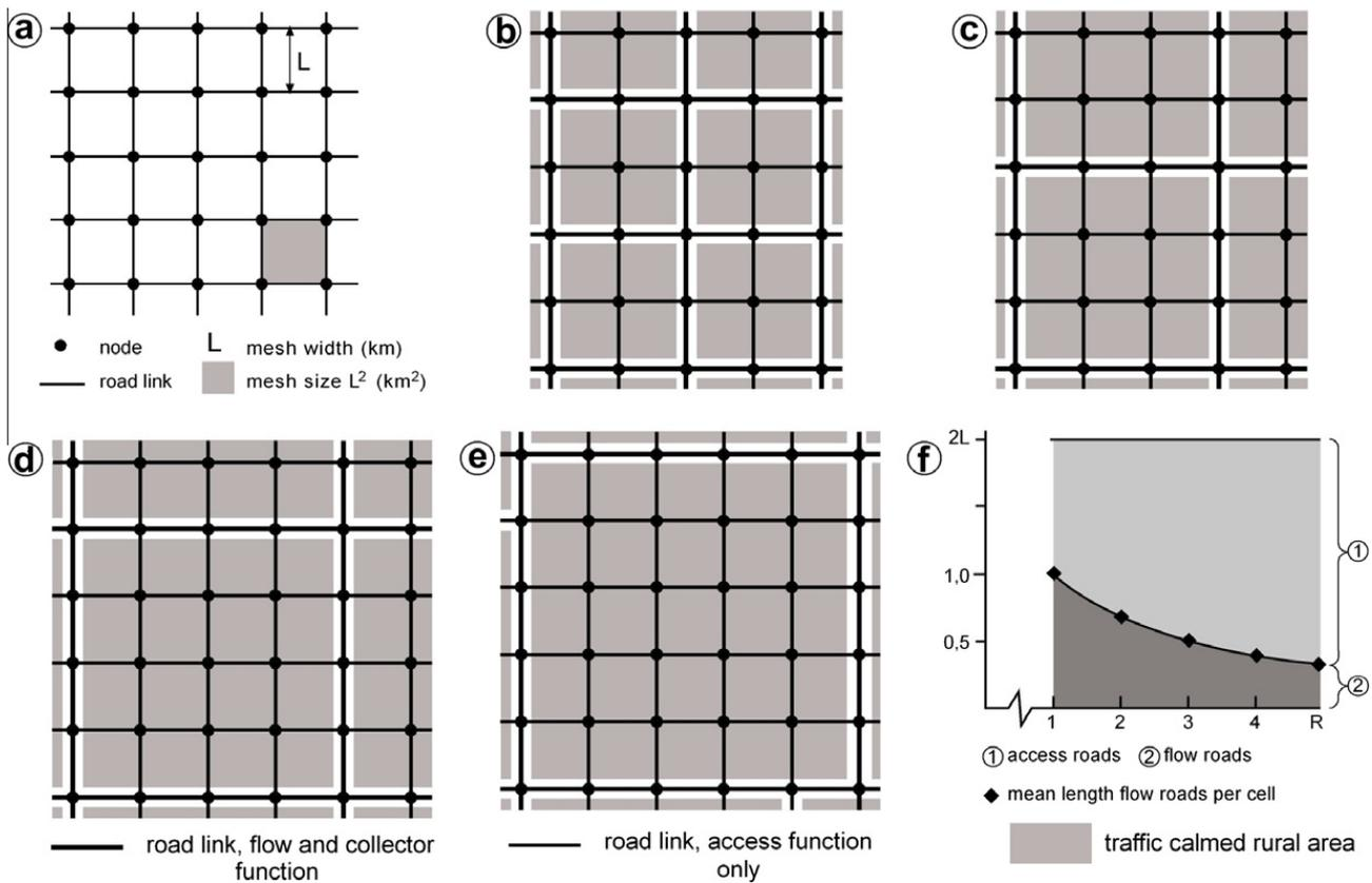
**Fig. 1.** Rural road networks in a regular square grid: (a) minor roads with nodes and road links with a length of  $L$  km; (b–e) two types of roads and sizes of the traffic-calmed areas; (f) the changing proportion of roads with access and flow function within the road length per grid cell ( $2L$ ) as function of the different sizes of the traffic-calmed area, as presented in (b) to (e).
