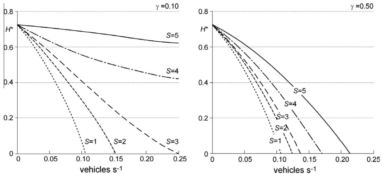
Fig. 4. Fraction of occupied patches  $H^*$  of 25 patches as function of the average traffic volume of all roads for different sizes of the traffic-calmed area.
